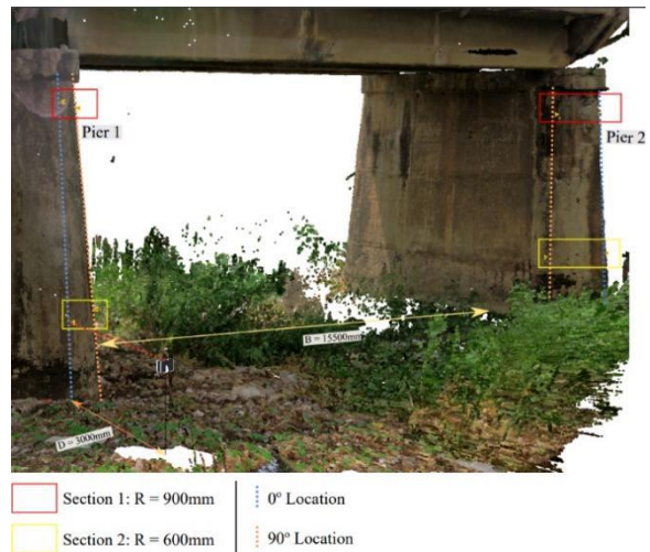
Figure 11. Measurement of point cloud interpoint spacing a h , at each location of the pier section
